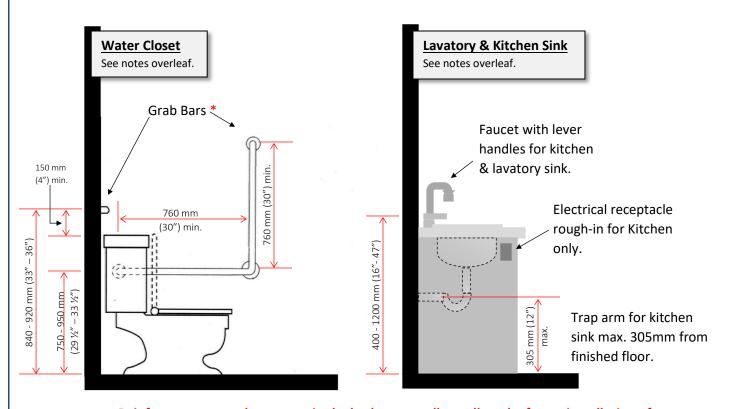
Reinforcement must be present in the bathroom walls to allow the future installation of Barrier Free grab bars as indicated for the water closet, shower and bathtub.
