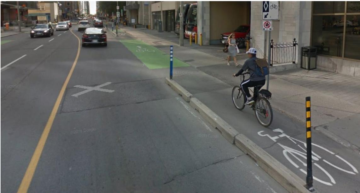
Figure 5 - Example of high-visibility paint markings used to denote a conflict area at a driveway in Ottawa, ON (from Google Maps)
