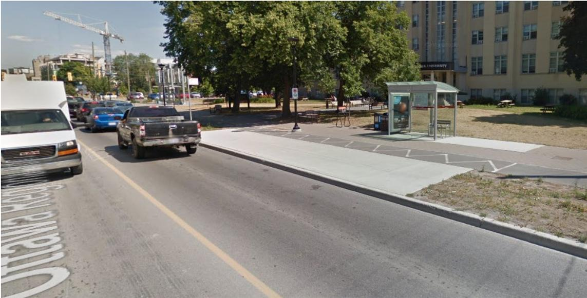
Figure 16 - Curb-side bus stop with cycle track running behind in Ottawa, ON (from Google Maps)
