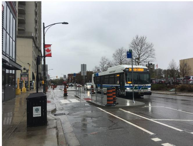
Figure 13 - Physically separated bicycle lane with bus islands in London, ON
