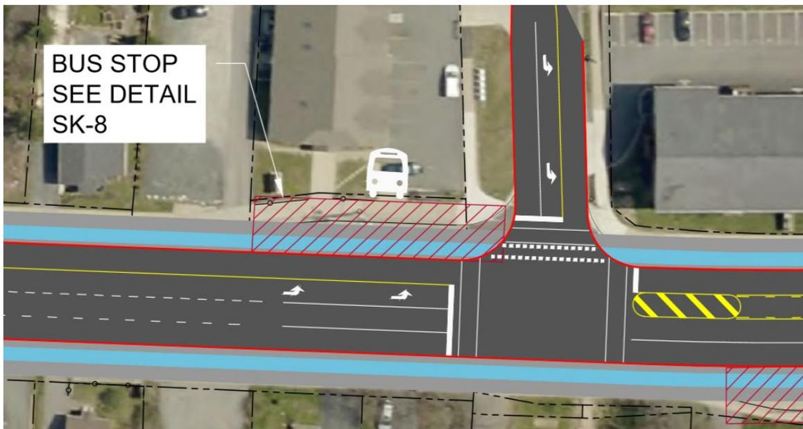
Figure 19 - Illustration of new signalized intersection at Drysdale Avenue in the ultimate scenario
