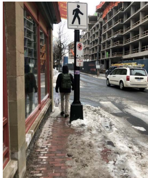
Figure 11: Pedestrian Pinch Point, West Side of Lower Water Street at Prince Street (75cm at Narrowest Point)
