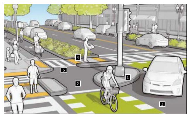
Figure 2.3.1- Protected Bikeway Intersection (Source: MassDOT)
