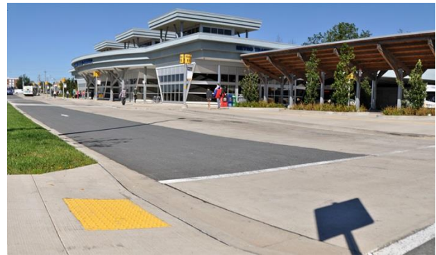
Tactile Markings at the Bridge Terminal
